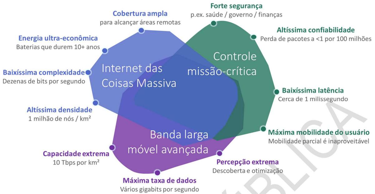
Fonte: Qualcomm. *Paving the path to narrowband 5G with LTE IoT*
